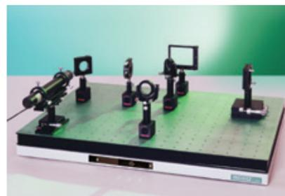
The AET Series is a series of desktop vibration isolators that bring together an entire high-performance vibration isolation system. At Meiritz Seiki, many of our previous desktop vibration isolators have been combined into a series. As a result, the AET Series, which combines these vibration isolators with steel honeycomb surfaces tables, consists of desktop air suspension vibration isolators are optimal for optical experiments using a small surface area.
